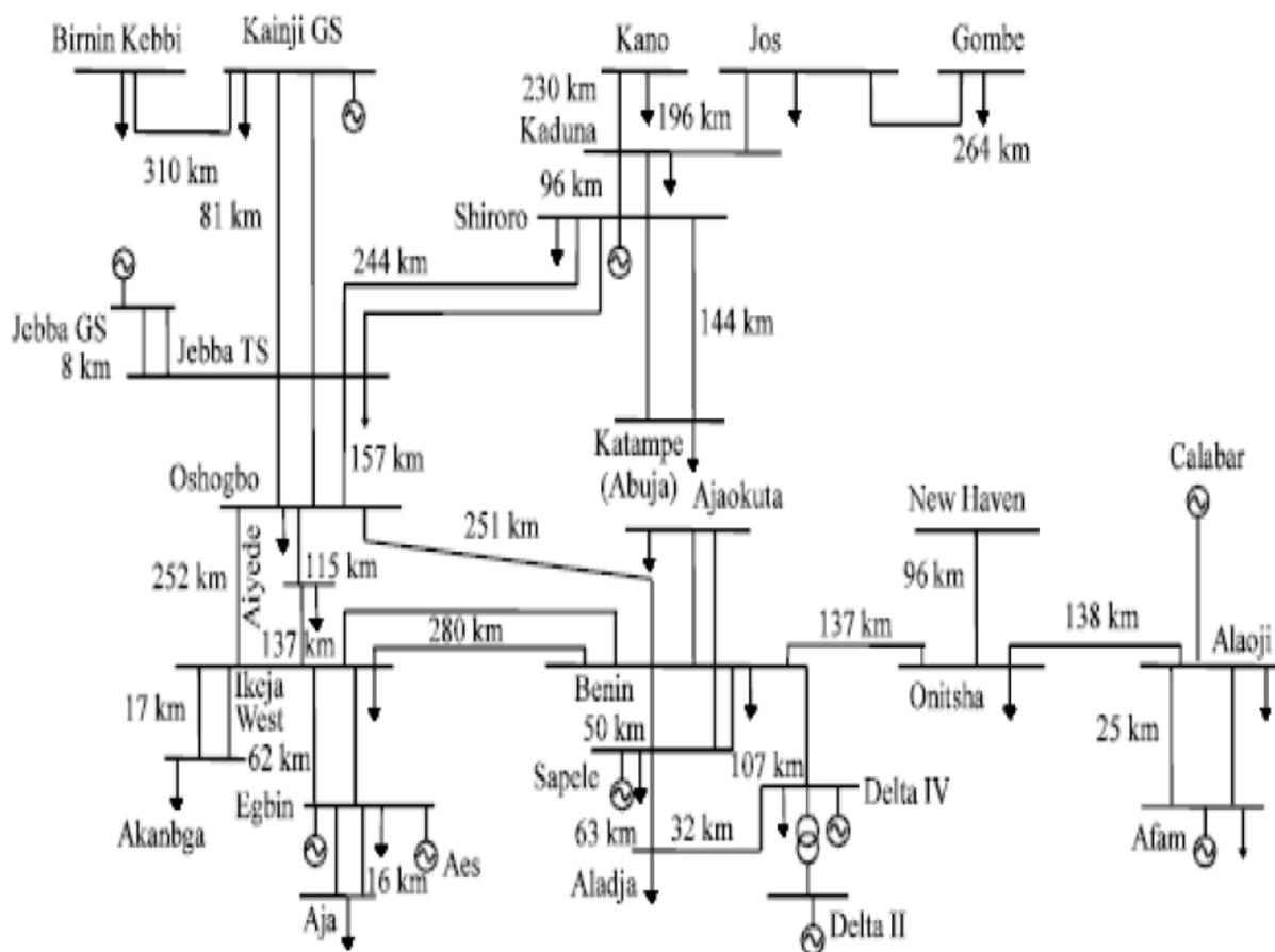
Fig 1: One-line diagram of Nigerian 330-kV transmission network [4]
